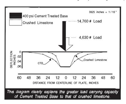
Notice that Cement Treated Base will support a significantly greater load than limestone and will distribute the load over twice the area. With superior load-bearing capacity and durability, CTB reduces the point-load impact on the subbase.
